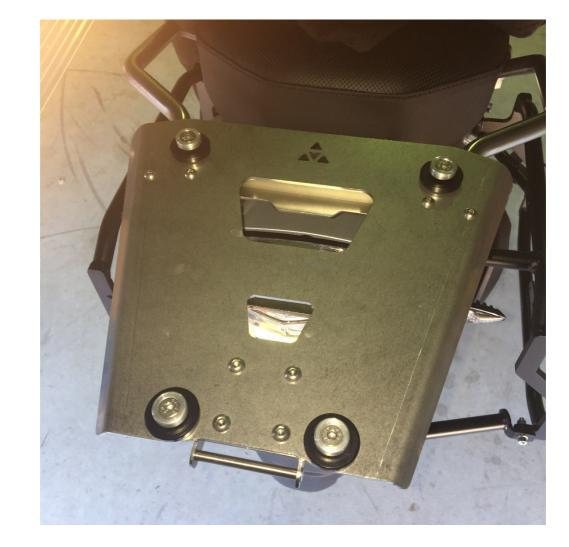
4. Tighten the four rear 6mm cap screws with nyloc nuts and then tighten the four front 5mm cap screws.
