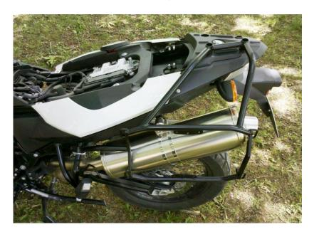
3. Attach the rack on the left side left foot peg mount as shown in photo with following hardware: 2 x Clamp, 2 x washer M5, 2 x screw M 5x35
