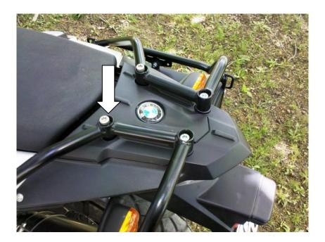
5. Fit rear connection bar as shown in the photo. Tighten all bolts.
