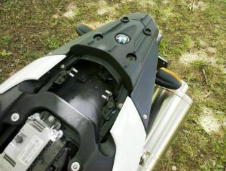
2. Start installation with the left side. Do not tighten bolt.
