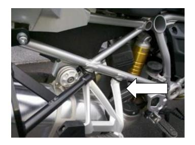
6. Attach the pannier frame to the bracket with 2 bolts M8 x 20.
