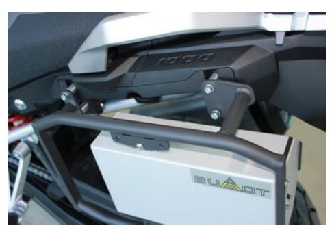
4. Attach the forward mounting point of the rack on the left side as shown in photo. Use the 4mm spacer in the forward mounting hole between the pillion peg bracket and the frame, and reattach the pillion peg bracket to the bike using the included M8 x 40mm bolts.
