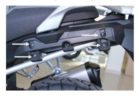
2. Remove the two bolts that attach the pillion peg bracket and remove the assembly.
