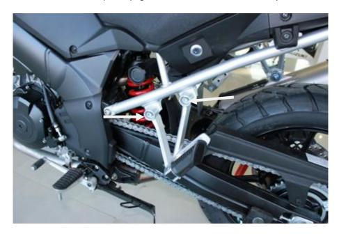
3. Attach the left side pannier rack to the frame with the included M6 x 40mm bolts, M6 washers, and spacers. Two 20mm spacers are used in the upper mounting points and two 23mm spacers are used in the lower mounting points.
