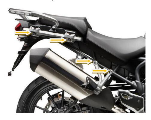
2. Using M8 x 50mm bolts, M8 washers and aluminium spacers, 15mm x 20mm as shown on the picture below.
