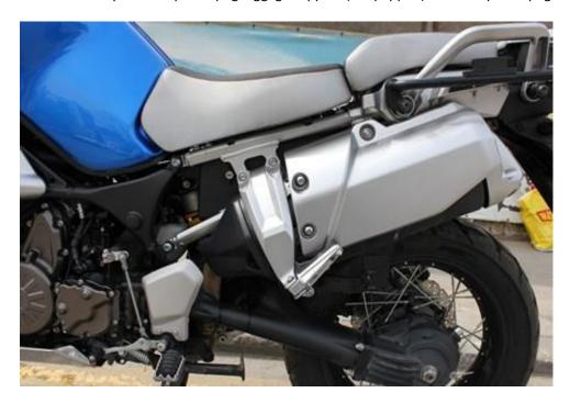
4. Attach the right side pannier rack to the frame with the included M10 x 80mm bolt, M10 washer, and 28mm spacer in the rear mounting point. Use the included M10 x 80mm bolt, M10 washer, and 15.5mm spacer in the front mounting point. Both spacers should be placed on top of the original Yamaha mount washer and behind the pannier rack mount. See picture below for hardware order.
