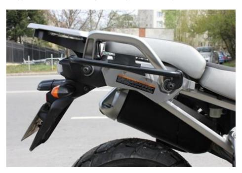
2. Remove the right side factory Yamaha pillion peg luggage support (if equipped) from the pillion peg bracket. Remove the two mounting screws and the pillion peg mounting bracket.
