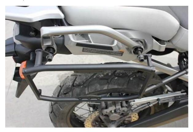
5. Install the pillion peg bracket over the BUMOT rack mount. Reinstall using the original bolts.
