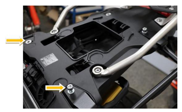
7. Attach the Pannier racks using M8 x 40 mm with 2 x washers M8 as shown on the picture:
