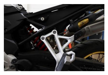
4. Put the aluminum spacers  $\phi$ 19 x 5mm as shown on the picture:
