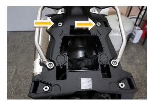
5. Put aluminum spacers  $\phi$ 19 x 9 mm as shown on the picture:
