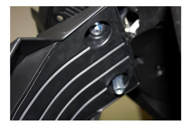
8. Attach the mud guard with the OEM bolts as shown on the picture. Tight them.
