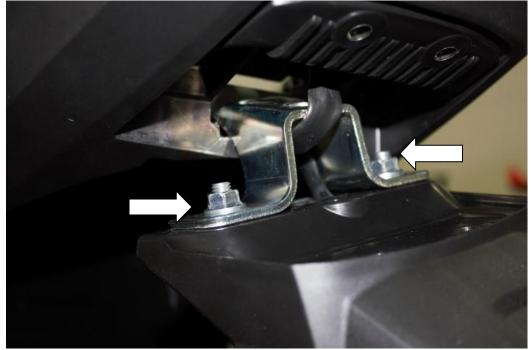
• Put the **External M8 x 20 mm Bolt** on the top of the bracket and M8 Nut 24mm under the mud guard as shown on the picture . Apply liquid threadlock (LocTite 243) and tight them
