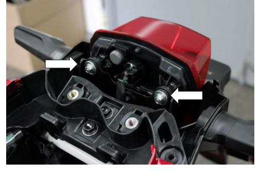
Remove the tail light - Rotate it up and pull
