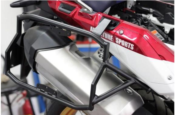
12. Attach the passenger foot pegs with OEM bolts and spacer 4mm as shown on the picture . Still do not tight them.
