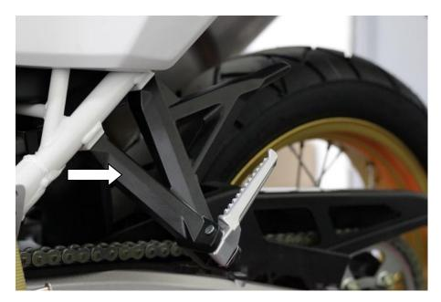
3. Remove the four bolts and grab handle as shown on the picture
