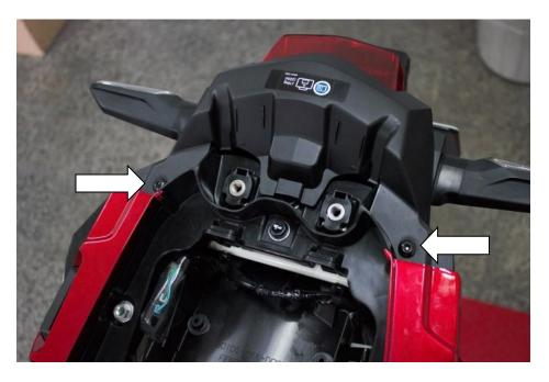
5. Disconnect the plug from the tail light and remove the two nuts and head washers as shown on the picture
