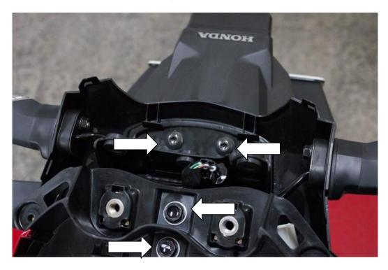
7. Remove the two bolts under the mud guard and two nuts as shown on the picture
