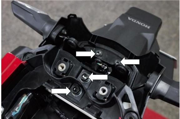
Mount the tail light and plastic cover on the top of the tail. Mount the grab handle on the bike.
