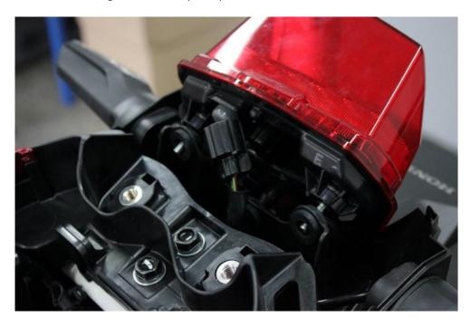
6. Remove the four bolts as shown on the picture.
