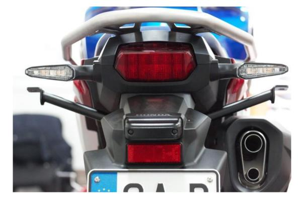
9. Attach the upper cross bar with **Inner head hex M8 x 16mm** Bolts .Keep the <u>right bolt</u> untighten as shown on the picture . The <u>left bolt</u> will be added as soon as the left frame is attached.
