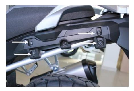
2. Remove the two bolts that attach the passenger peg bracket and remove the assembly.
