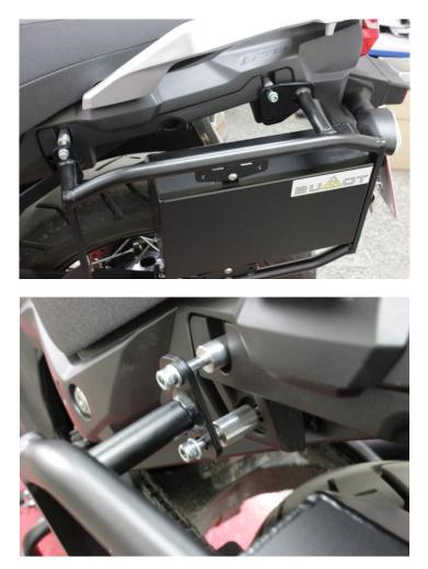
4. Attach the forward mounting point of the rack on the left side as shown in photo. Use the 4mm spacer in the forward mounting hole between the passenger peg bracket and the frame, and reattach the passenger peg bracket to the bike using the OEM M8 bolts.
