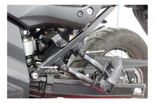
3. Attach the left side pannier rack to the frame with the included M6 x 40mm bolts, M6 washers, and spacers. Two 20mm spacers are used in the upper mounting points and two 23mm spacers are used in the lower mounting points.
