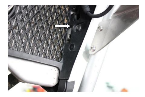
5. Attach the left and right rad guards with the two OEM bolts M6x25 as showed on the picture:
