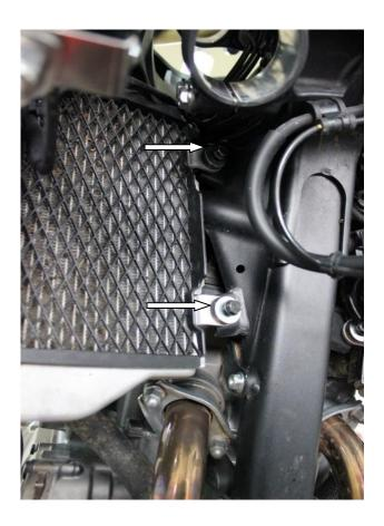
2. Remove the three OEM bolts and washers.
