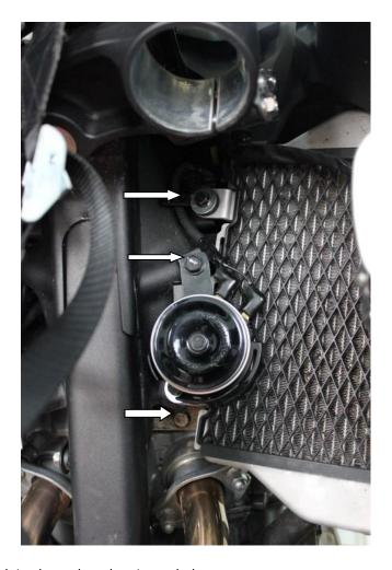
3. Remove the screw which is showed on the picture below:
