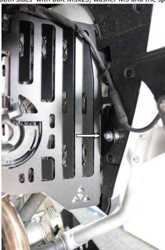
7. Attach the horn with Bolt M8x20 and 2 x M8 washers as showed on the picture below:
