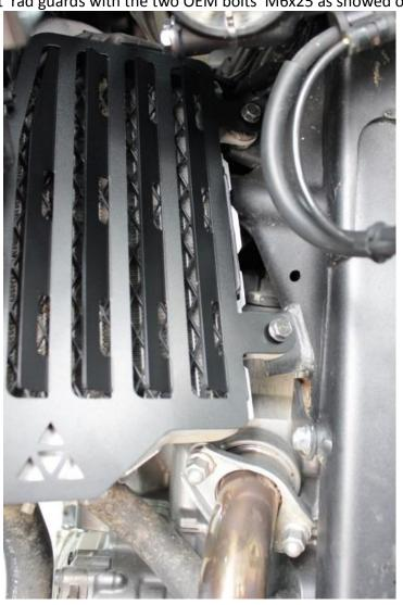
6. Attach the rad guards on both sides with bolt M5x25, washer M5 and the spacer M10 :
