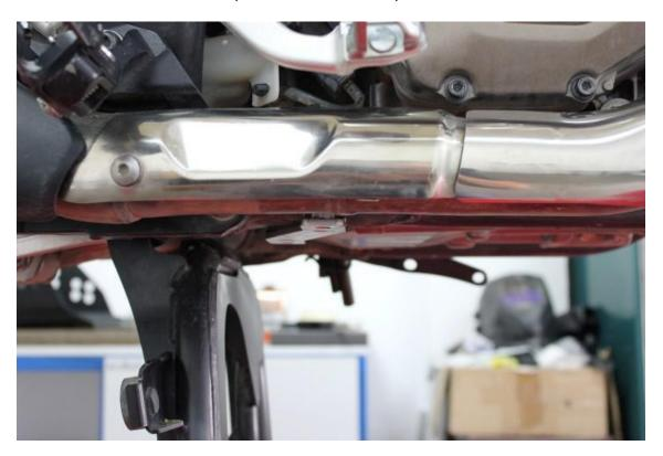
6. Use M8x50 Bolts and M8 Finish washers to attach skid plate to the bike. Do not tighten them yet, leave a 1mm gap.
