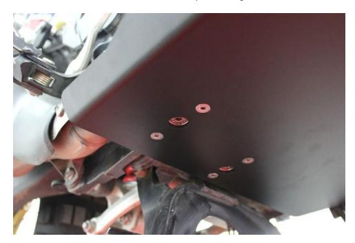
9. Tighten the front bolts M8x50 and the two OEM ones.
