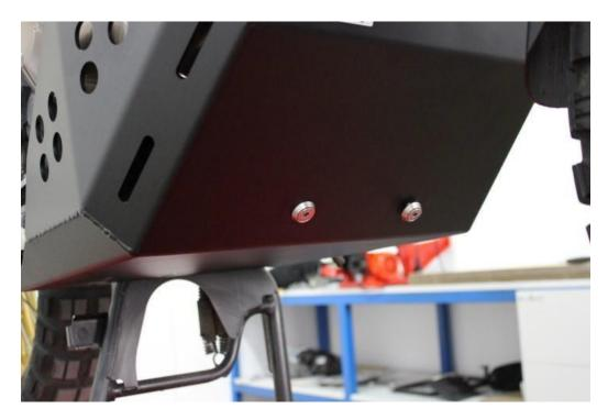
7. Attach the skid plate bracket using two OEM bolts as shown on the picture. Do not tighten them yet!
