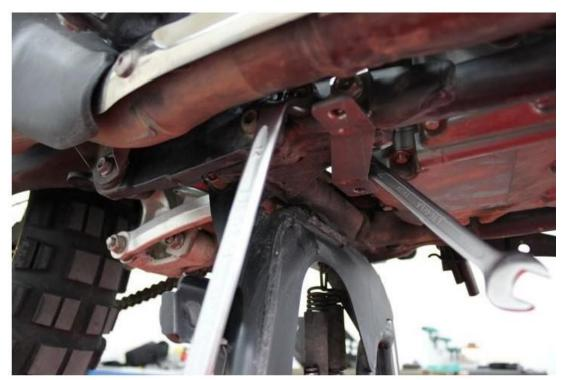
The bracket has to be in horizontal position as shown on the picture!
