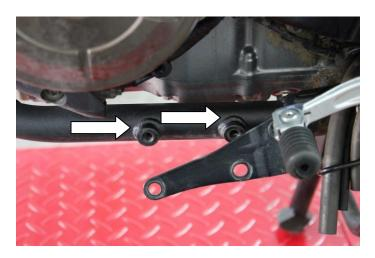
3. Remove the nut from the rear bolt (white arrow) and loosen the front nut (yellow arrow)
