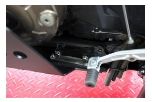
8. Use M8 x 16 bolts to attach the bottom of skid plate and tighten them.
