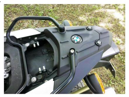
2. Remove the plastic caps and remove the original 4 bolts on the tail.
