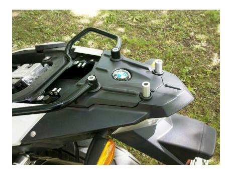
4. Attach the top racks using 4 x M8x50 and tighten.
