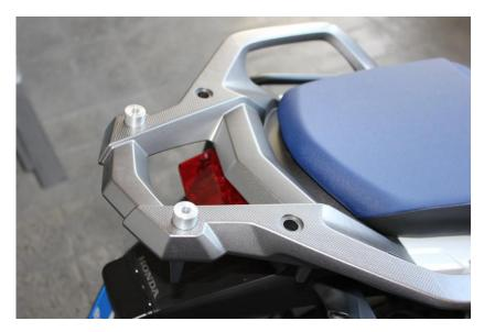
2. Install the top case mounting plate and the four bolts as shown on the picture below.
