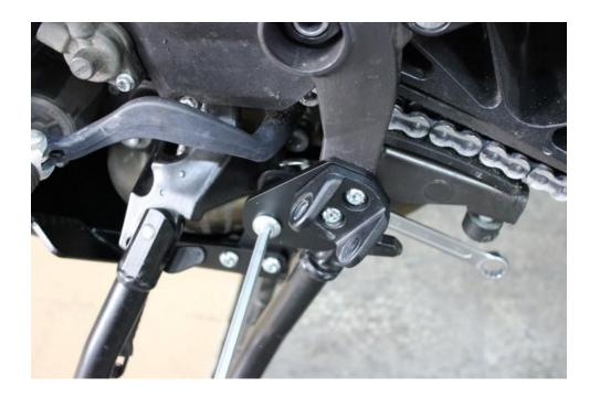
8. Attach the front side of the skid plate using bolt M10x80 from the left and right side as shown on the picture. Use thread locker. Tight all bolts!
