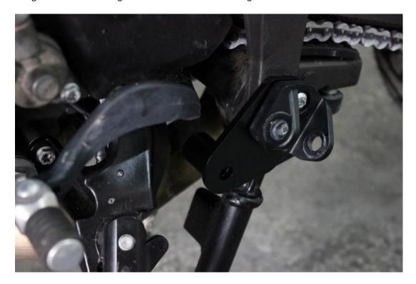
6. Use the 17 mm spacer on the left side and the 22 mm spacer on the right side.
