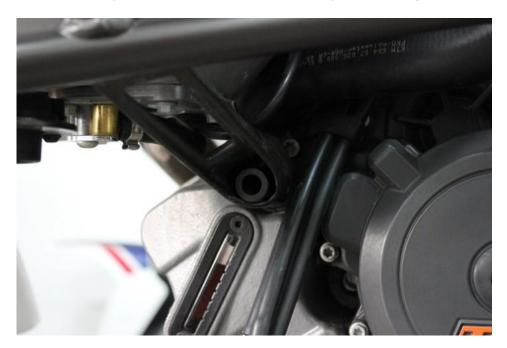
7. Attach the rear side of the skid plate using M10x50 Button Head Bolt and M10 nut on both sides. Do not tight the bolts yet.
