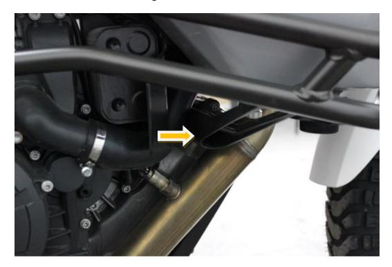
5. Attach the bracket and foot peg mount as shown on the pictures with two bolts M8x20 Button head bolts using thread locker and tight them. Do the same on the right side.
