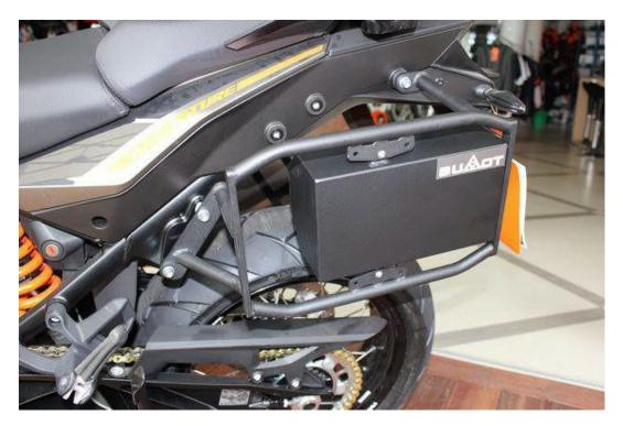
4. Install the right side pannier rack to the frame by starting with the lower mounting bracket. In the mounting hole at the front of the lower bracket, use a M8 x 50mm bolt, a M8 washer, and the original aluminum spacer. In the mounting hole at the rear of the lower bracket, use a M8 x 70mm bolt, a M8 washer, and the included 22mm aluminum spacer. The smaller diameter of the included spacer should be on the bike side.
