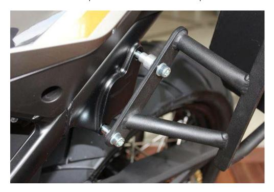
3. Install the upper mounting point of the left side rack with a M8 x 20mm bolt and M8 washer.
