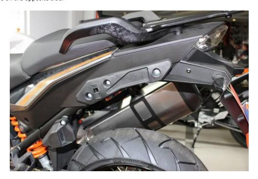
2. Install the left side pannier rack to the frame by starting with the lower mounting bracket. In the mounting hole at the front of the lower bracket, use a M8 x 35mm bolt, a M8 washer, and the original aluminum spacer. In the mounting hole at the rear of the lower bracket, use a M8 x 50mm bolt, a M8 washer, and the included 22mm aluminum spacer. The smaller diameter of the included spacer should be on the bike side. See picture below for detail.
